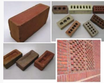
Exposed Cored (with holes)
