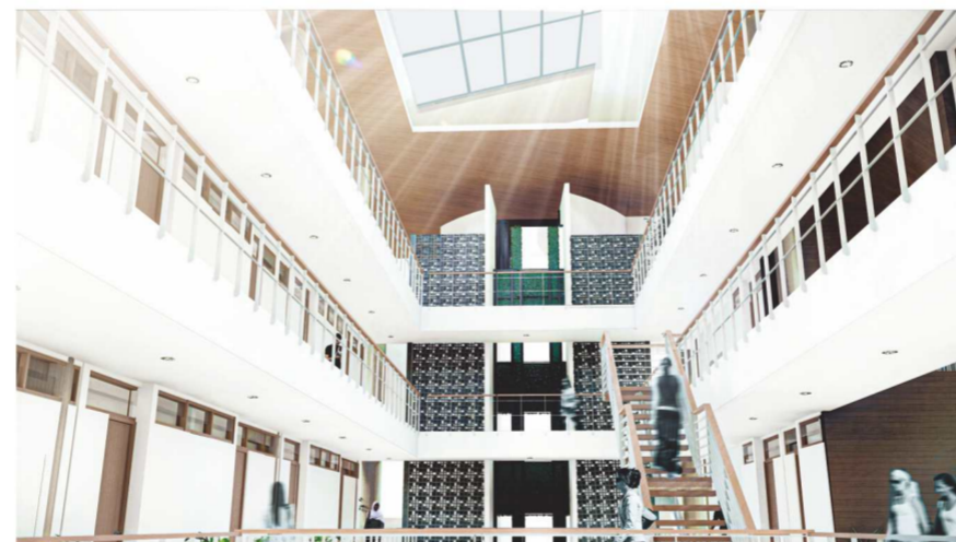
The skylight features in the roof ensure abundant natural light and promote air circulation, ensuring proper ventilation in the corridors and bedroom units.
